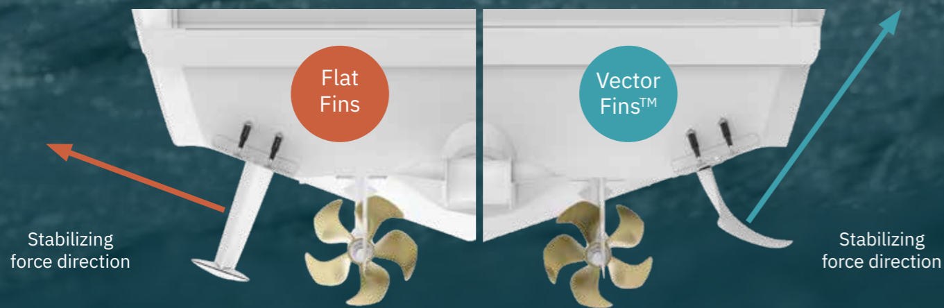
This simplified illustration shows how the Vector Fins™ better directs the fin forces toward the desired vertical direction, minimizing the energy waste of too many forces being used in the horizontal plane, which can cause unwanted side effects such as yaw and sway.
