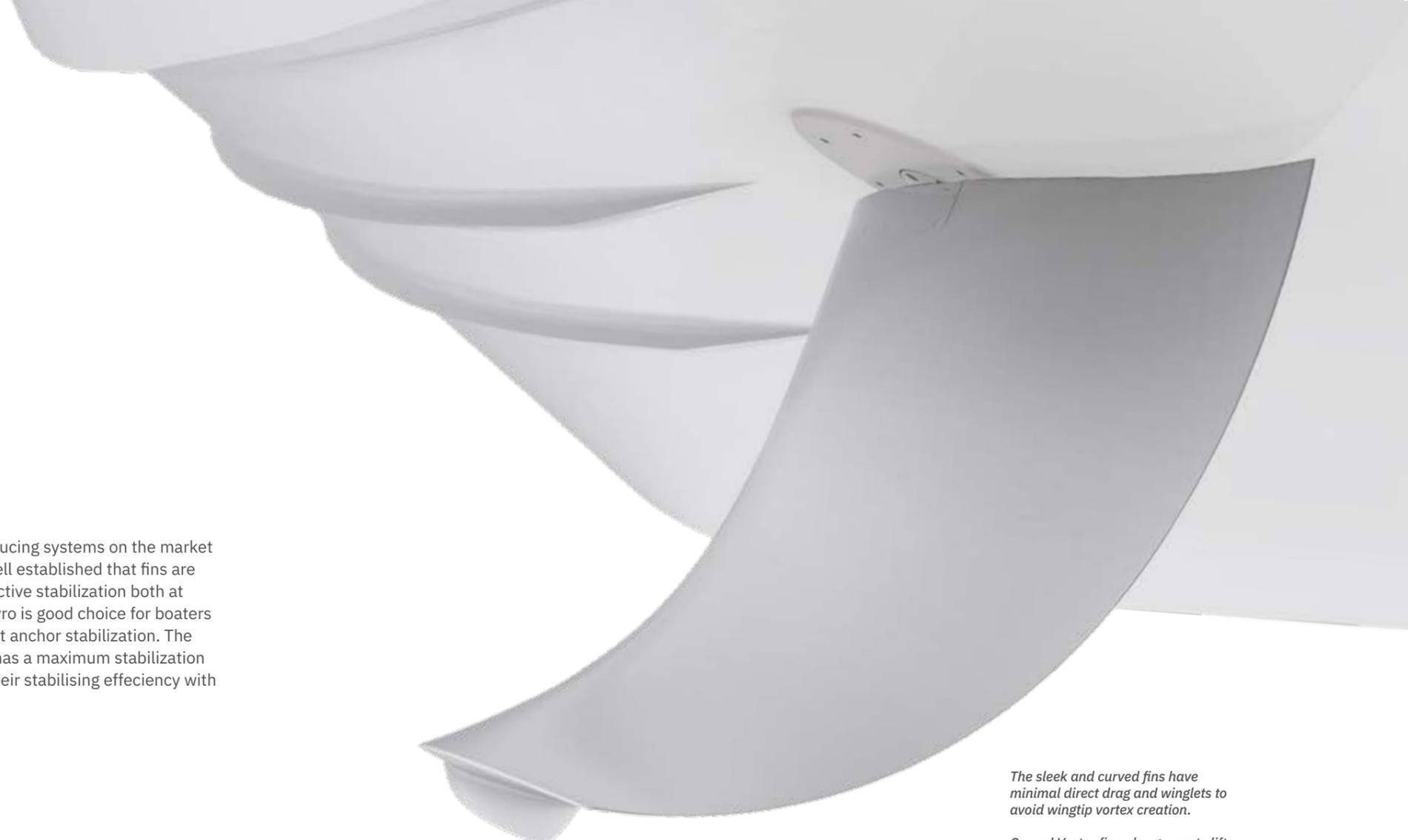
*The sleek and curved fins have minimal direct drag and winglets to avoid wingtip vortex creation.*
