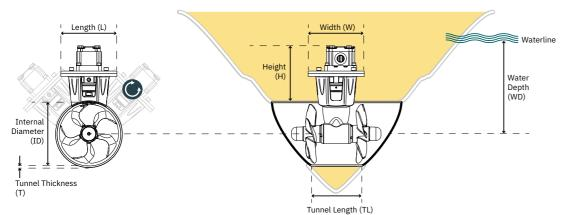
Sleipner thrusters can be installed at an angle off the vertical centre. Tailored to fit any space available in your vessel.
