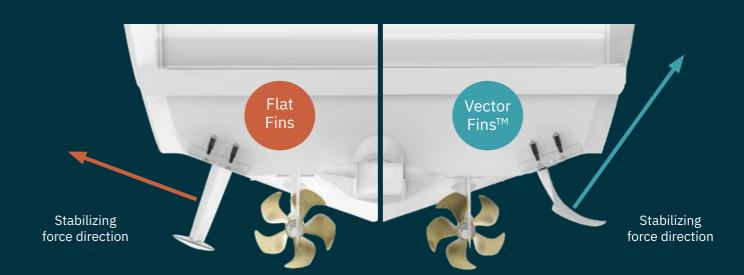
This simplified illustration shows how the Vector Fins™ better directs the fin forces toward the desired vertical direction, minimizing the energy waste of too many forces being used in the horizontal plane, which can cause unwanted side effects such as yaw and sway.
