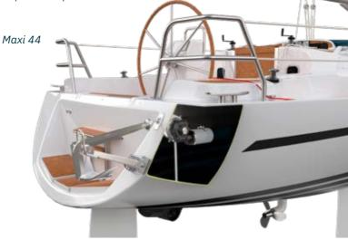
With the Maxi 43 and 44, you can decide which side you want to install the line wheel. We recommend having the line wheel facing towards the middle of your vessel instead of out towards the hull. This will allow easier access for service and maintenance. However, this depends on your boat's construction and your preferences.
