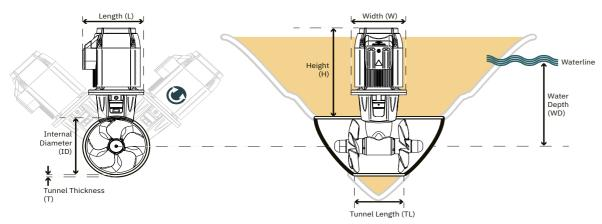
Sleipner thrusters can be installed at an angle off the vertical centre. Tailored to fit any space available in your vessel.
