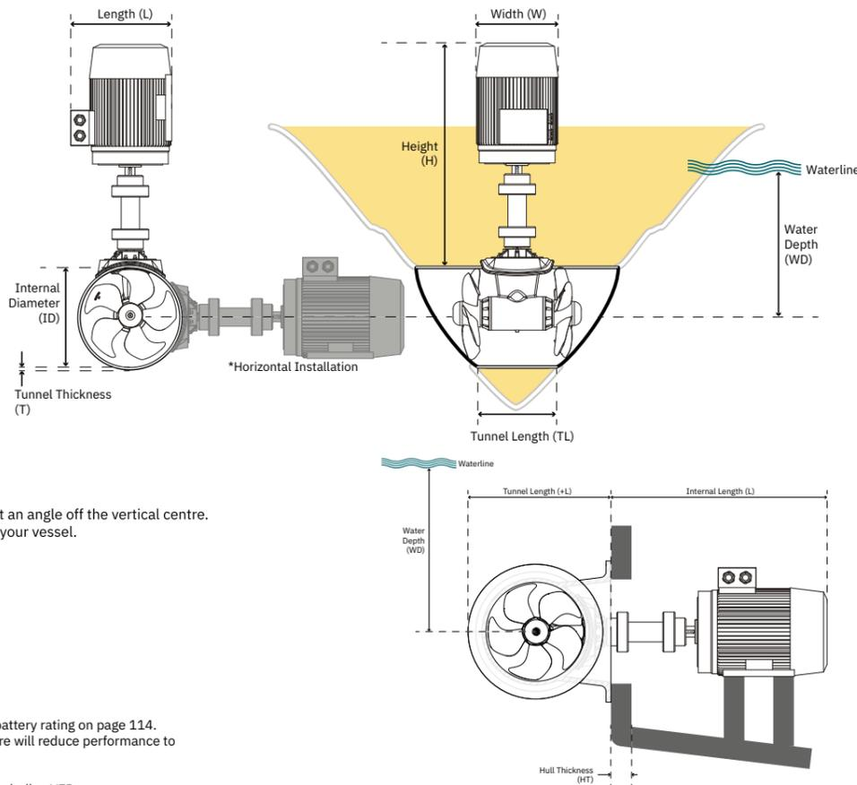
Sleipner thrusters can be installed at an angle off the vertical centre. Tailored to fit any space available in your vessel.
