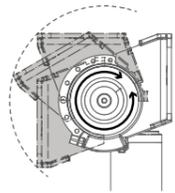
\* The Windlass system is designed to allow customizable orientation of the motor or support bracket. Offering for more flexibility to install the windlass system in the space you have available.
