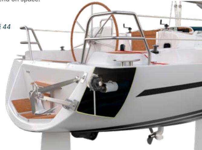
With the Maxi 43 and 44, you can decide which side you want to install the line wheel. We recommend having the line wheel facing towards the middle of your vessel instead of out towards the hull. This will allow easier access for service and maintenance. However, this depends on your boat's construction and your preferences.
