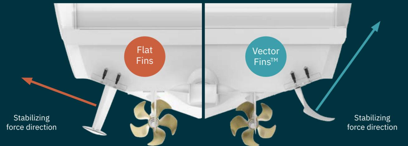
This simplified illustration shows how the Vector Fins™ better directs the fin forces toward the desired vertical direction, minimizing the energy waste of too many forces being used in the horizontal plane, which can cause unwanted side effects such as yaw and sway.
