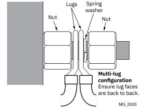
placed in the outer position before tightening nut.
