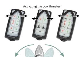
Activating both bow and stern thruster to push the boat sideways
