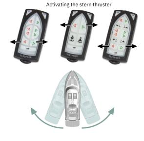
Activating both bow and stern thruster to rotate the boat on axis
