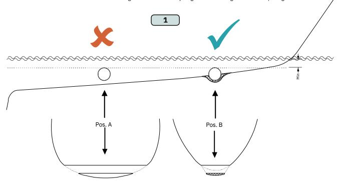
1. A possible problem in sail boats or fast powerboats is that a non-rounded surface can generate drag from the back face of the tunnel, as it creates a "flat" area facing the flow of water.
