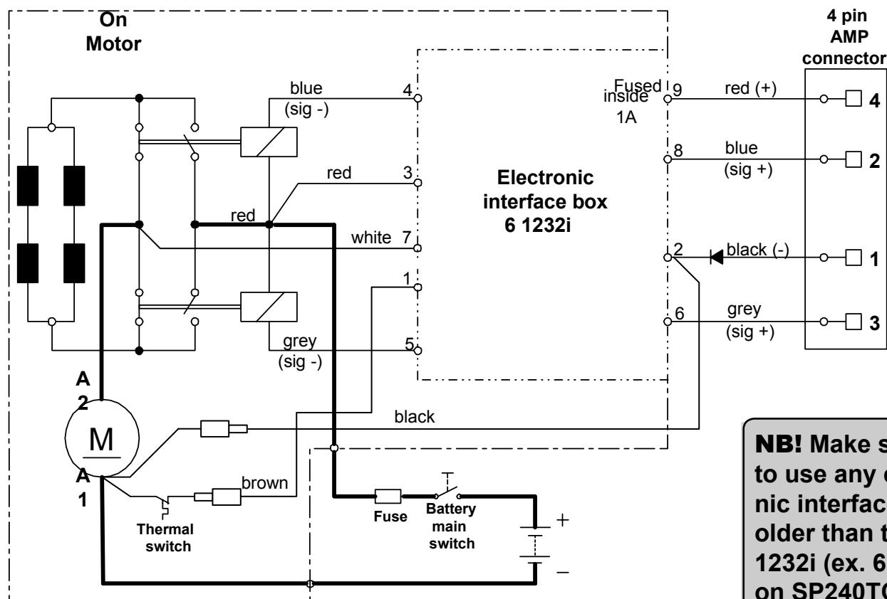
**The SP 285 TCi is a 48V thruster and will therefore need some extra installation parts in a boat with a 24V electrical system.**
